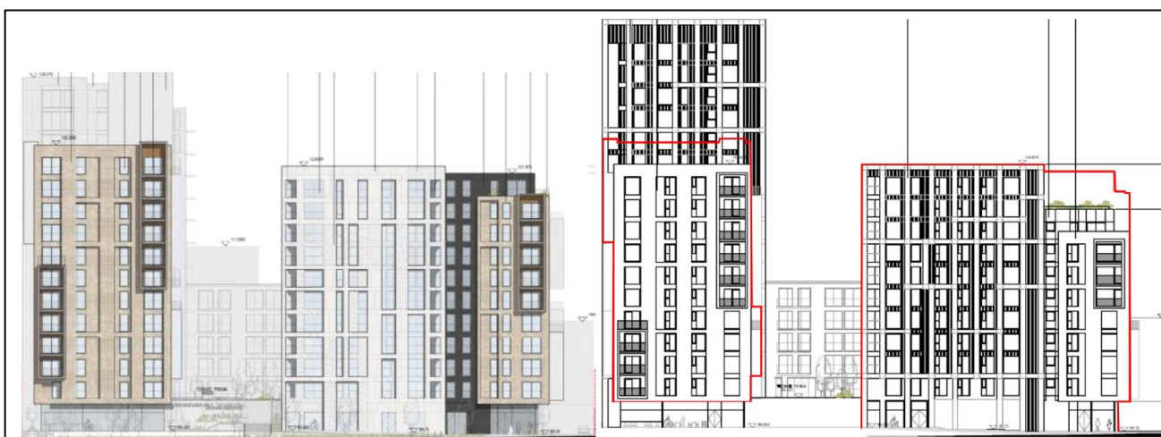
Figure 3.13: Contextual north-east elevation of the alternative design as submitted for pre-application consultation (Left), and revised Proposed Development design for the current application (Right). The red line indicates the comparable outline of the pre-application consultation design.
